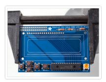
Flip over the PCB and solder in the three legs of the potentiometer
