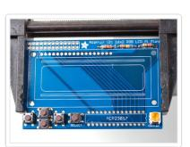
Flip over the PCB and check that all the legs for the buttons are sticking out.
