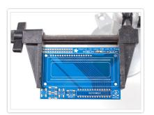
Put the printed circuit board into a vise or board holder, heat up your soldering iron and make sure you're ready to go! We'll start with the first resistor **GREEN** which has orange, orange, brown, gold bands on it. This resistor acts as the backlight control resistor for the green backlight pin.
